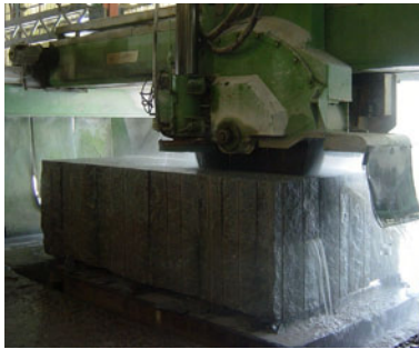
Granite block cut with disc
