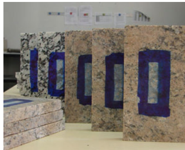
Marks of erosion by abrasion in the abrasion test
